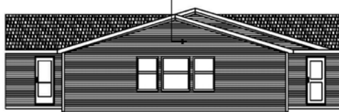
Figure 40. (Right) Tag unit offset roof connection
